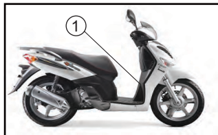
Vehicle identification number ( VIN )
